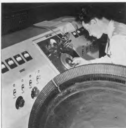
FIGURE 1. TYPE 713-B Beat-Frequency Oscillator mounted in assembly with power amplifier.
