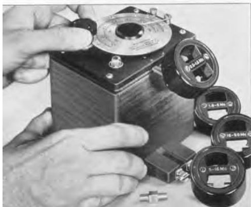
FIGURE 3. View of the TYPE 566-A Wavemeter in use. The coil can be rotated to secure optimum coupling to the source whose frequency is being measured.
