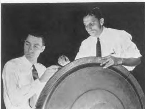
FIGURE 3 (above). Engineers move the crystal pickup along the bucket tips. The pickup output is fed to the cathode-ray oscillograph shown below.
