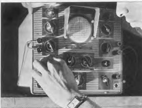
FIGURE 4 (below). Points of peak vibration are noted on the oscillograph as the pickup is moved along the buckets.
