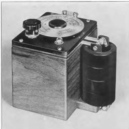
FIGURE 1. View of the TYPE 566-A Wavemeter showing how coils are stored when not in use.
