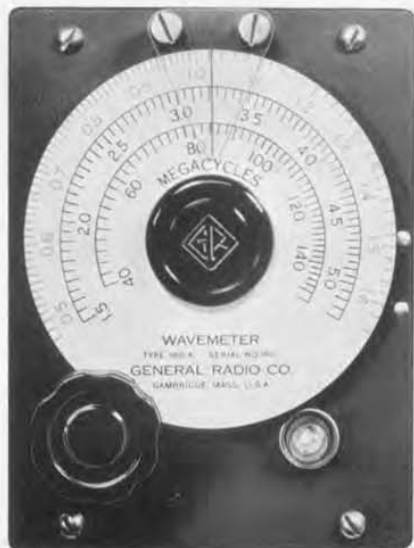
FIGURE 2. View of the wavemeter dial showing the frequency scales. The outer scale is engraved in red, the other two in black.
