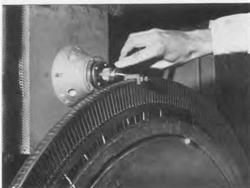
FIGURE 2. The oscillator supplies power to vibrate the turbine buckets through a power amplifier and an electro-mechanical transducer shown above.
